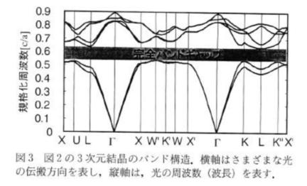
規格化周波数 Normalized frequency 図 3 図 2 の 3 次元結晶のバンド構造,横軸はさまざまな光の伝搬方向を表し, 縦軸は,光の周波数(波長)を表す。 Figure 3: Band structure of 3D crystal of Figure 2; the horizontal axis represents various propagating direction of light, and the vertical axis represents frequency (wavelength) of light
